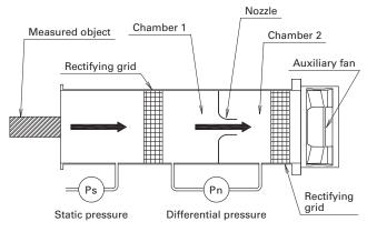
Fig. 3: Model diagram of the Airflow Tester
