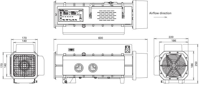
Fig. 2: Dimensions of the "San Ace Airflow Tester"
