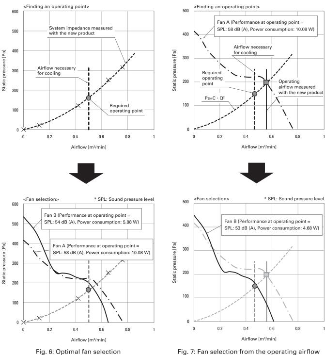
from the system impedance of a device
